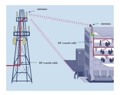
The following diagram illustrates the application of leaky coaxial cables:
