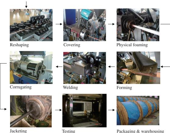
It generally takes about 200 minutes to produce one kilometre RF coaxial cables from reshaping to packaging.
