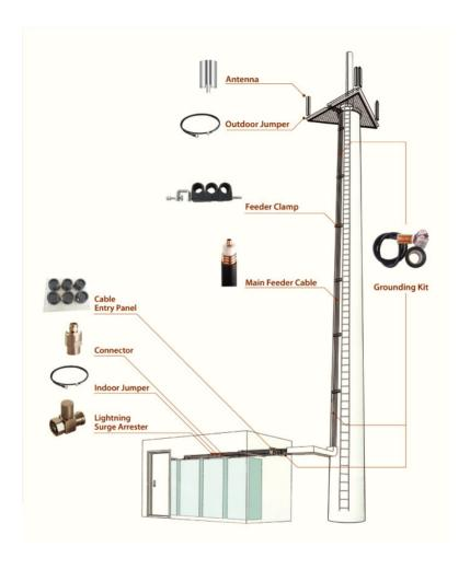
The following diagrams illustrate the application of RF coaxial cables:
